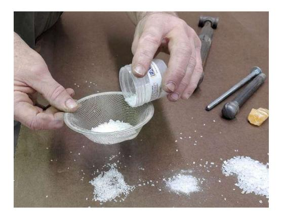
Crushed material can be purchased in various sizes, delineated by inches, mm, micron, or mesh screen, which can get quite confusing. Calibrated mesh screens can be quite expensive too and is a bit of an overkill for our needs. A simple method is to buy a kitchen sink drain screen. The one I have is about a 14 mesh / .05" and is perfect for sifting out finer bits. A flour sifter works well, too.
