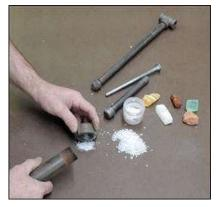
Use a 1" black pipe found at most hardware stores with an end cap for the mortar and (a small diameter black pipe with end cap or bolt that will fit inside the larger pipe for the ram (pestle). I have a large one for shell and minerals shown above and a smaller one for opal and finer minerals shown below.
