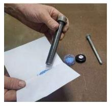
The smaller one is a 3/8" pipe with end cap and a 5/16" x 8" carriage bolt with the threads cut off and tip rounded smooth.
