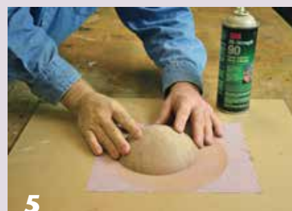
5 After waiting overnight, re-true the rim on a flat surface using 120-grit abrasive.
