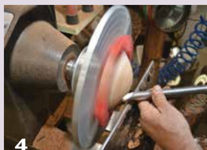
4 Rechuck using either large plate jaws or a vacuum chuck and complete the outside of the form to a rounded, footless bottom.
