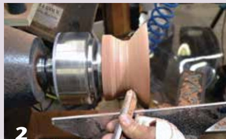
2 Shape as much of the outside of the vessel as your tool allows you to reach.
